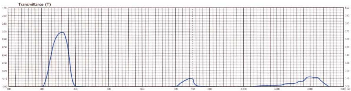
Figure 42. Transmission curve of HOYA U360 filter.
