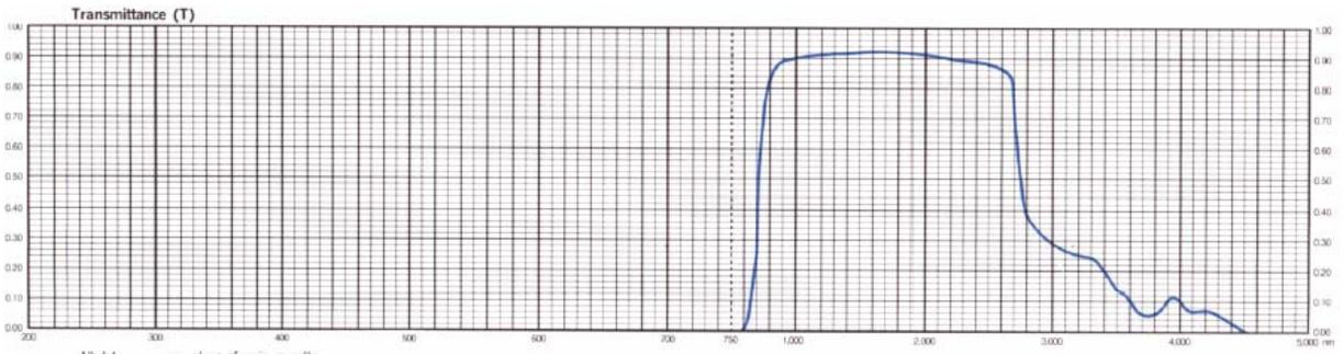
**Figure 44.** Transmission curve of HOYA IR85 filter.
