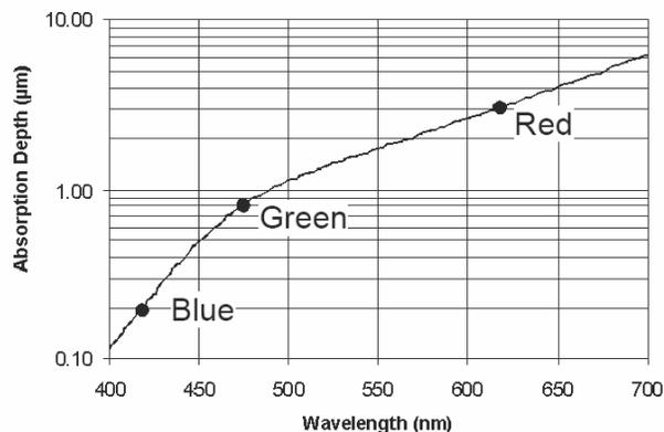
**Figure 2. Absorption Depth of Silicon with Wavelength. The photodetectors used in FOVEON camera are located at the three depths of 0.2 μm, 0.8 μm and 3 μm [4].**
