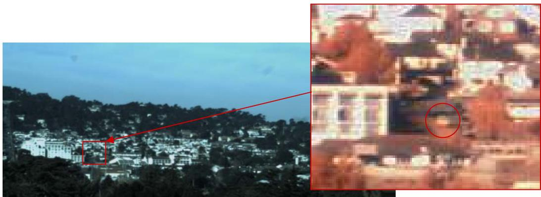
**Figure 26.** Image of downtown Monterey captured with the camera filter (400 nm to 660 nm) affixed. The zoomed-in image of a car is shown.
