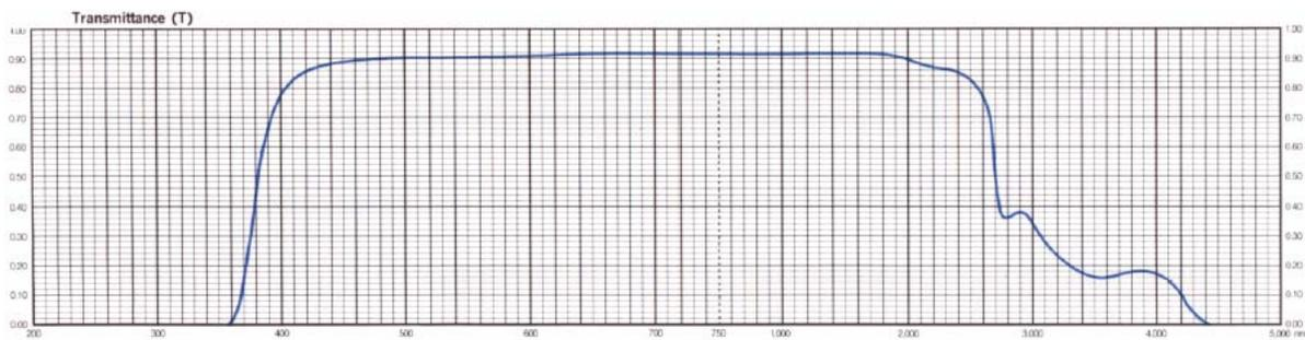
Figure 43. Transmission curve of HOYA L38 filter.
