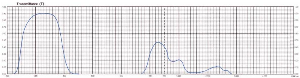
Figure 41. Transmission curve of HOYA U325C filter.
