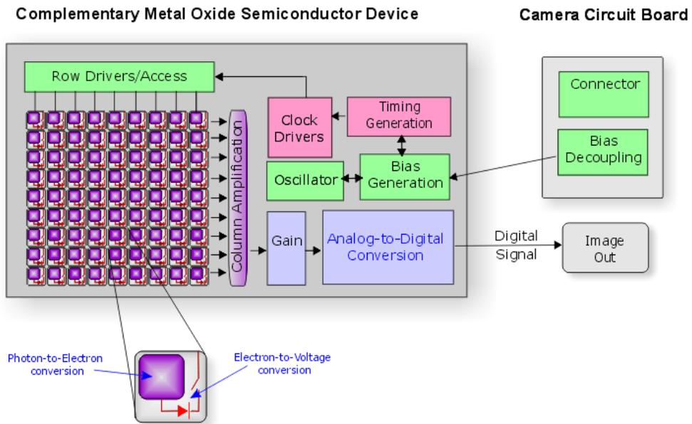
**Figure 23. Image Processing within a CMOS Sensor [14].**
