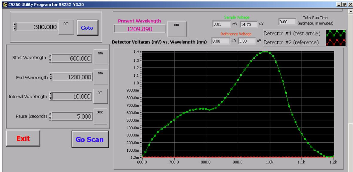
Figure 11. Screenshot of LabView Monochromator Control Program.
